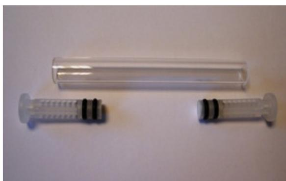
The **column body** (i.e. the tube) is made of acrylic. It has an appearance similar to a glass tube, i.e. clear and transparent.
